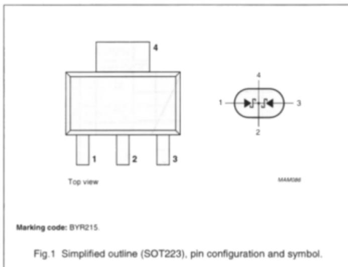
Fig.1 Simplified outline (SOT223), pin configuration and symbol.
