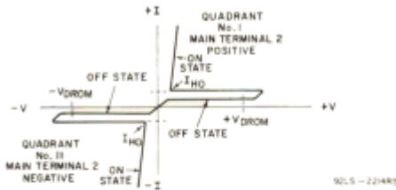
Fig. 1 - Principal voltage-current characteristic.
